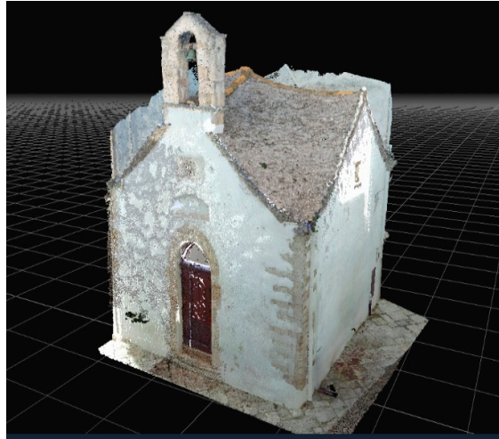
Figure 7. Three-dimensional (3D) point cloud of San Nicola in Montedoro.
