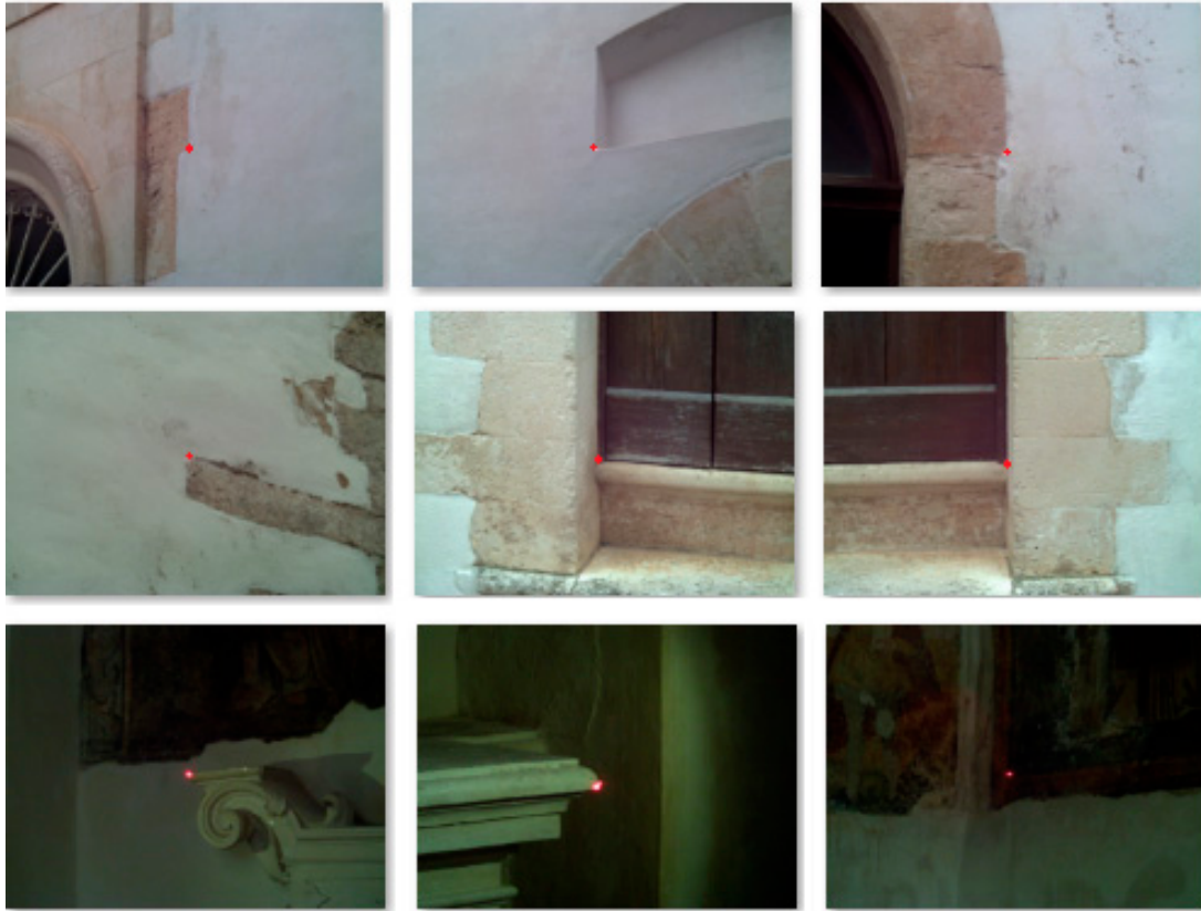
Figure 4. Images of some ground control points used for the georeferencing of the point cloud.
