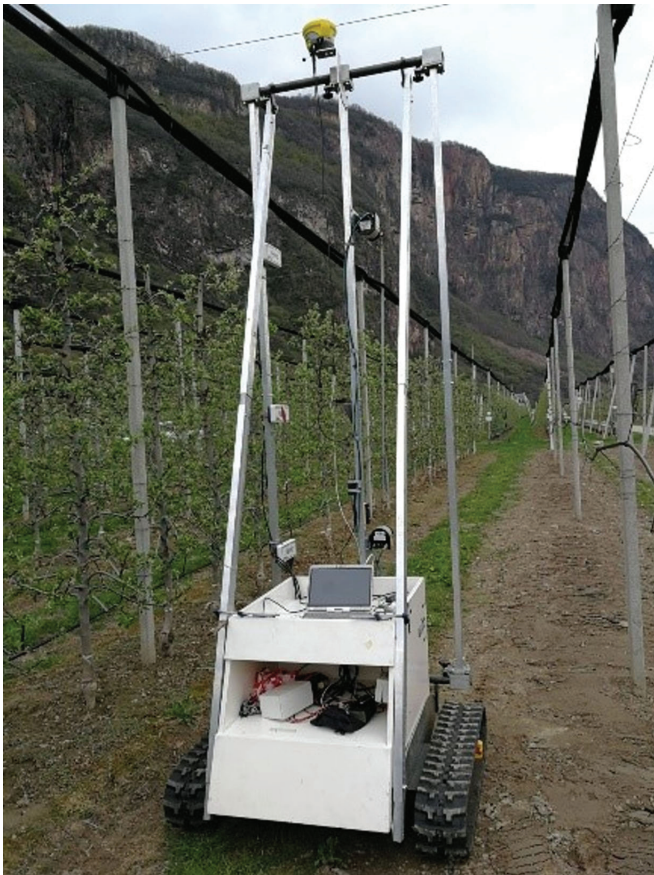
Figure 1. The figure shows the ByeLab used during the survey, the sensors mounted on the metal structure (on the left of the three OptRx™ sensors, on the central pole: (i) the GNSS receiver, (ii) the two LiDARs, and (iii) the IMU) and on the white structure the computer
