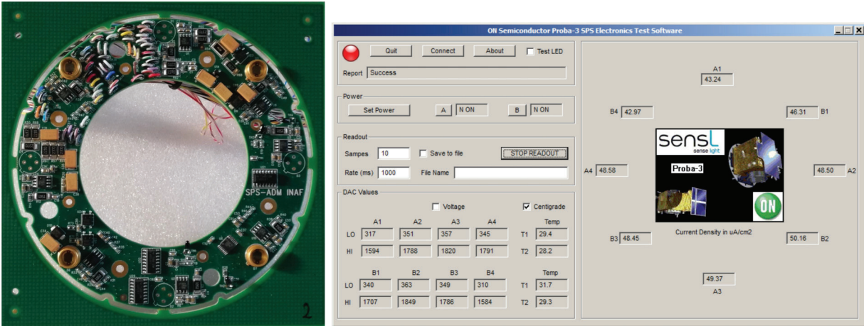
Figure 3. Advanced Demonstration Model of the SPS (the ADM with only 4 SiPMS mounted is shown in order to highlight the mounting electronics geometry).
