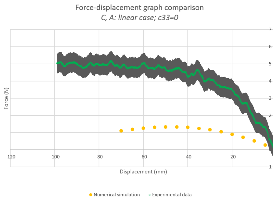
Figure 3. Numerical-experimental comparison—Specimen 1, not fitted ( c_{num} = c_{lin} , a_{num} = a_{lin} , c_{33} = 0 N/m). The grey area represents the error-type.
