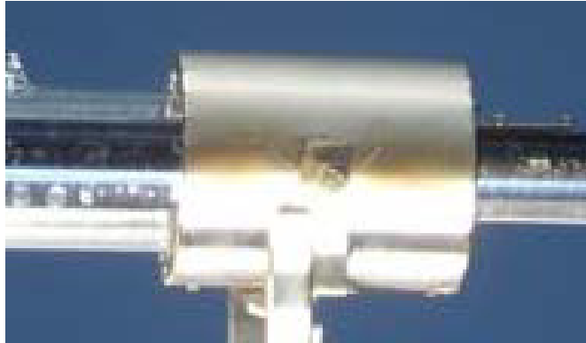
Fig. 6: the right receiver without the glass envelope, fully removed after the breaking event.
