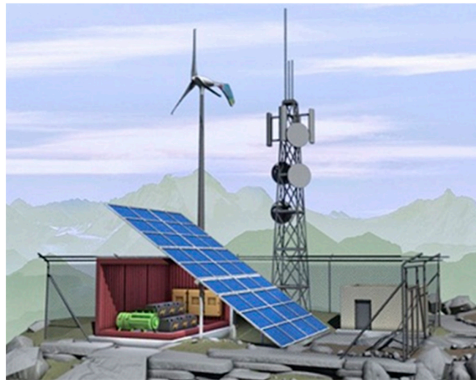
Figure 10. Possible site configuration based on HPS with PEMFC for Radio Networks in Mission-Critical Applications.
