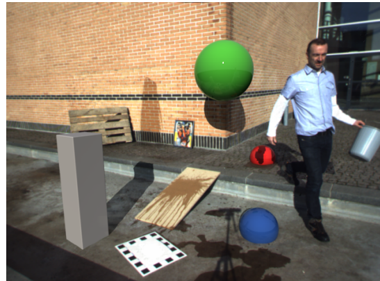
Figure 1: Frame 139 of a 200 frame sequence. The diffuse grey box and the three glossy spheres are rendered into the scene with illumination estimated from the shadow cast by the walking person.
