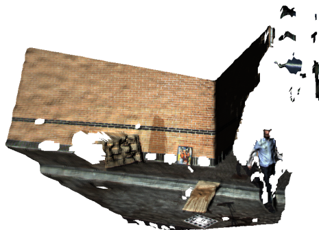
Figure 2: Textured 3D scene mesh generated from stereo disparity information from the image shown in figure 1. Notice how well the main surfaces in the scene are reconstructed.
