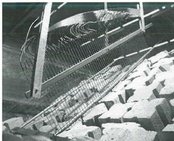
Figure 11: A novel step gauge for laboratory wave run-up measurements on a breakwater slope ( designed and constructed at Ghent University ).
