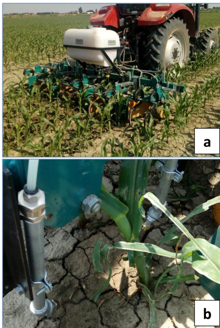
Figure 1. Treatment T1: Prototype of inter-row cultivator modified for band application of post-emergence herbicides (a) and detail of the two nozzles arranged to spray obliquely on a single crop row (b).
