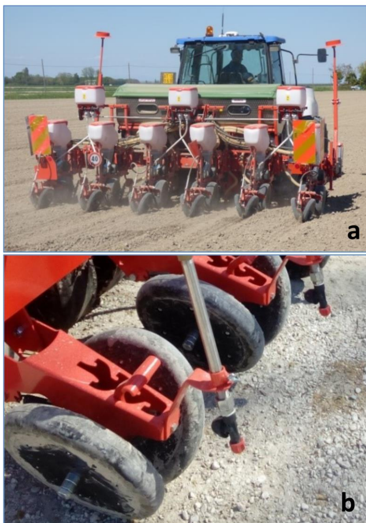
Figure 2. Treatment T2: 6 row maize seeder equipped for band application of pre-emergence herbicides (a) and detail of the nozzle arranged to spray along the single crop row (b).
