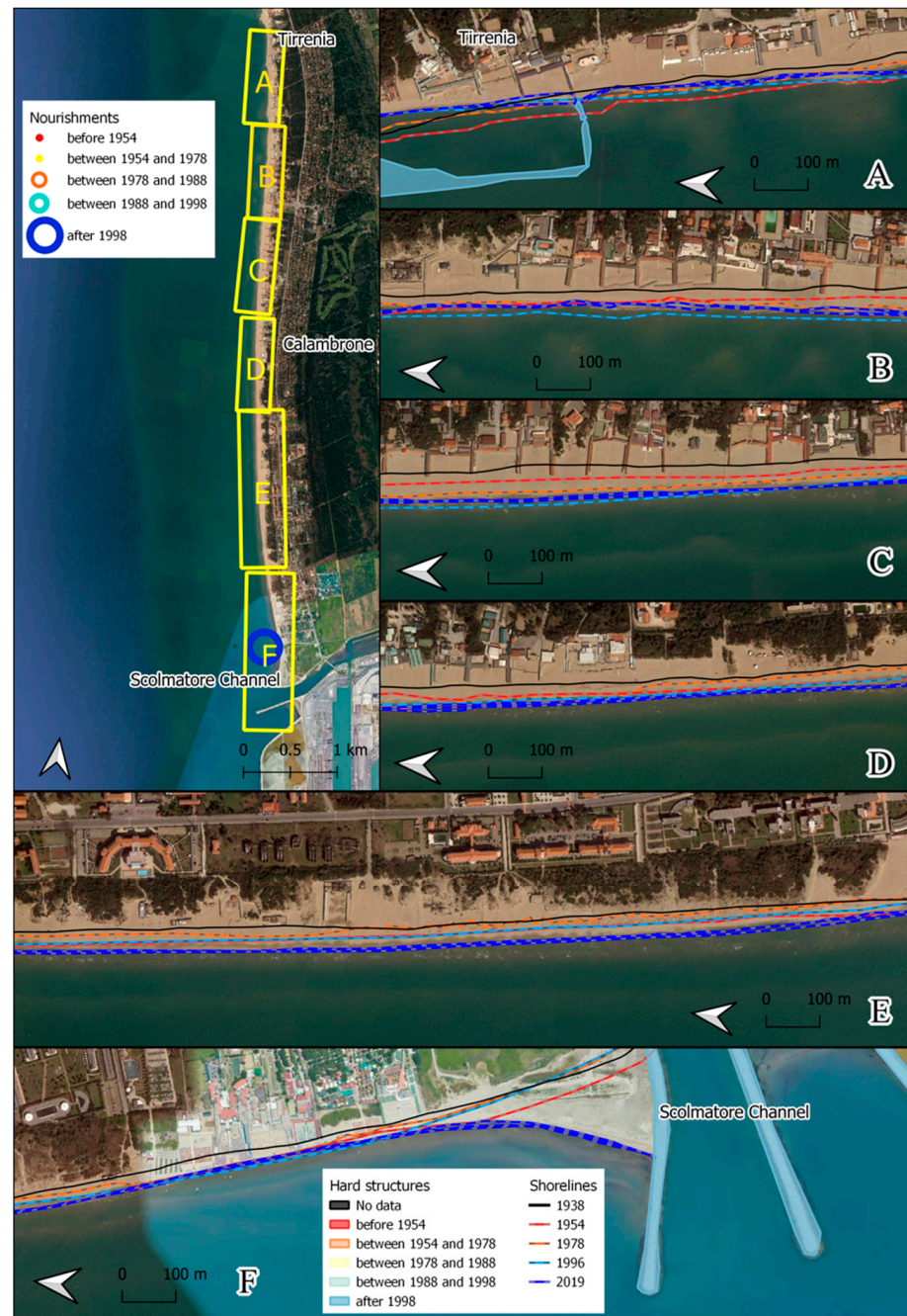
Figure 9. Identification of hard and soft operations along the sector comprised between Tirrenia and the Scolmatore Channel mouth. Polygons represent the hard structures; dots represent the nourishments. The yellow frames in the top left panel correspond to the zoom in panels to the right and at the bottom. The background image has been retrieved from the Google Earth database.
