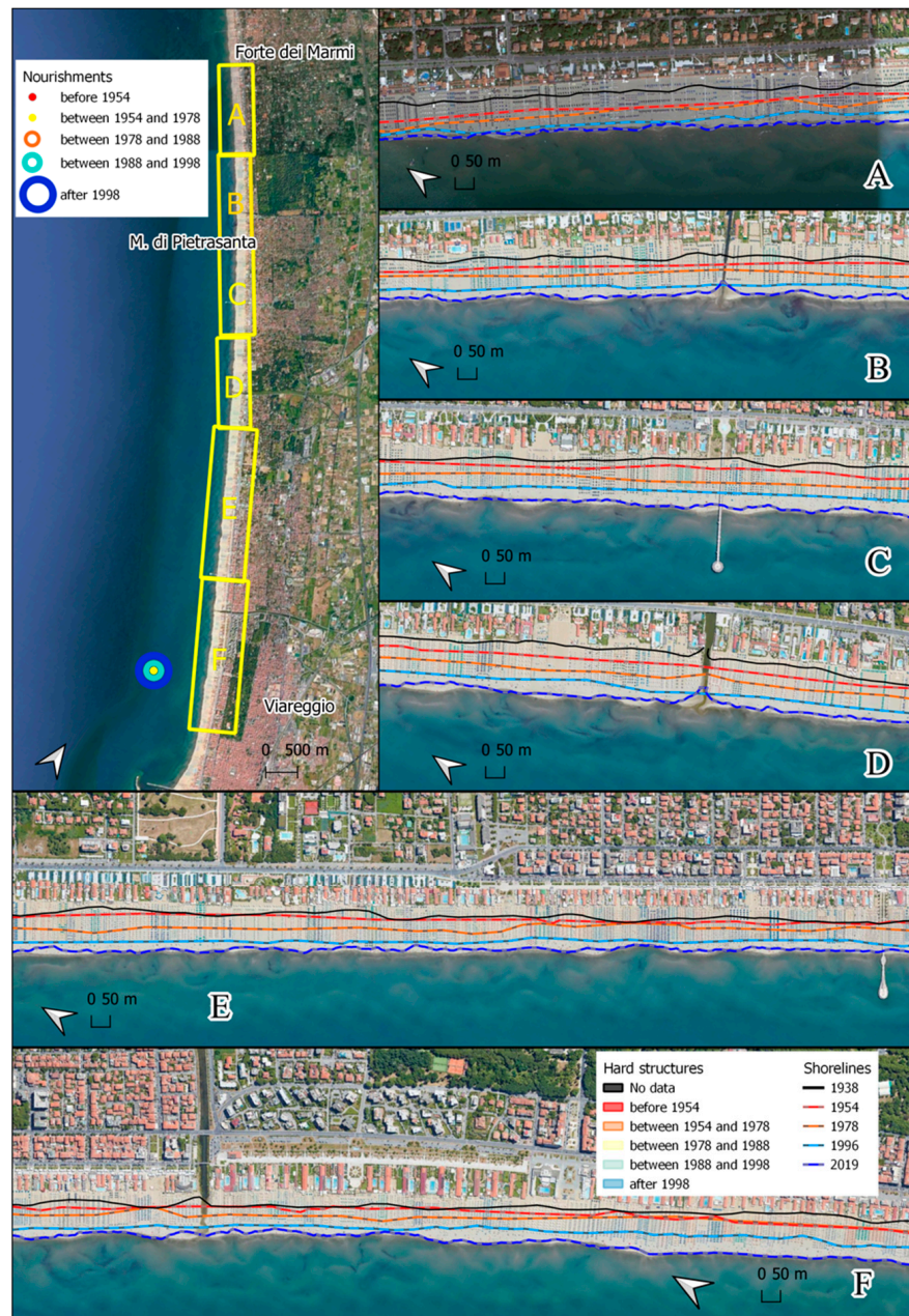
Figure 6. Identification of hard and soft operations along the sector comprised between Forte dei Marmi and Viareggio. Polygons represent the hard structures; dots represent the nourishments. The yellow frames in the top left panel correspond to the zoom in panels to the right and at the bottom. The background image has been retrieved from the Google Earth database.
