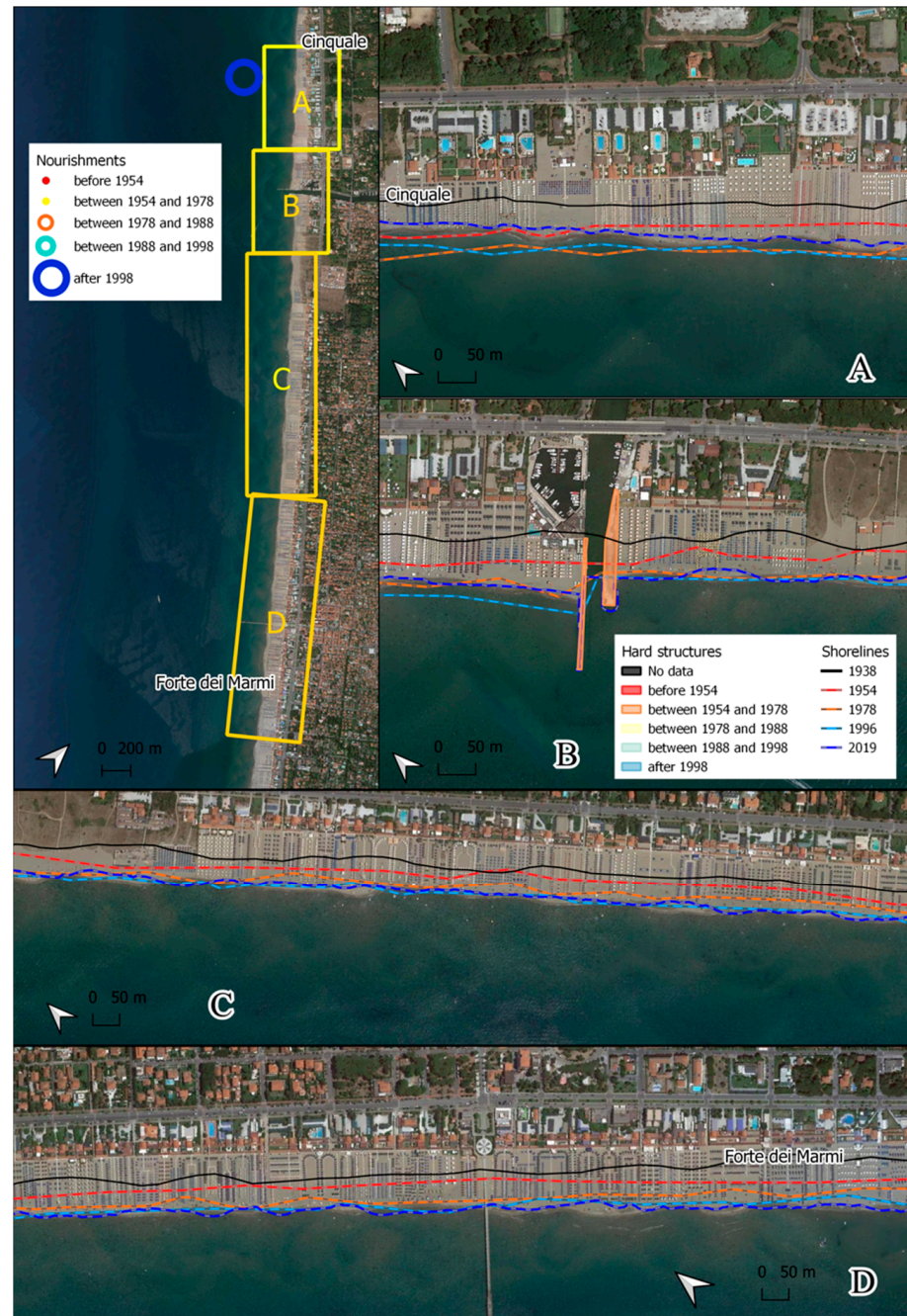
Figure 5. Identification of hard and soft operations along the sector comprised between Cinquale and Forte dei Marmi. Polygons represent the hard structures; dots represent the nourishments. The yellow frames in the top left panel correspond to the zoom in panels to the right and at the bottom. The background image has been retrieved from the Google Earth database.
