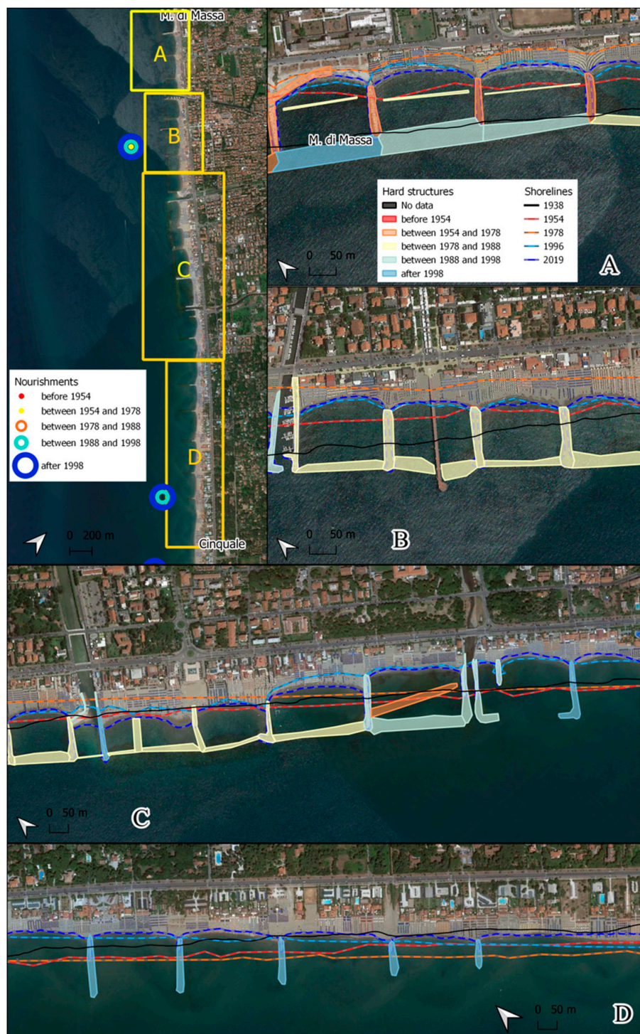
Figure 4. Identification of hard and soft operations along the sector comprised between Marina di Massa and Cinquale. Polygons represent the hard structures; dots represent the nourishments. The yellow frames in the top left panel correspond to the zoom in panels to the right and at the bottom. The background image has been retrieved from the Google Earth database.
