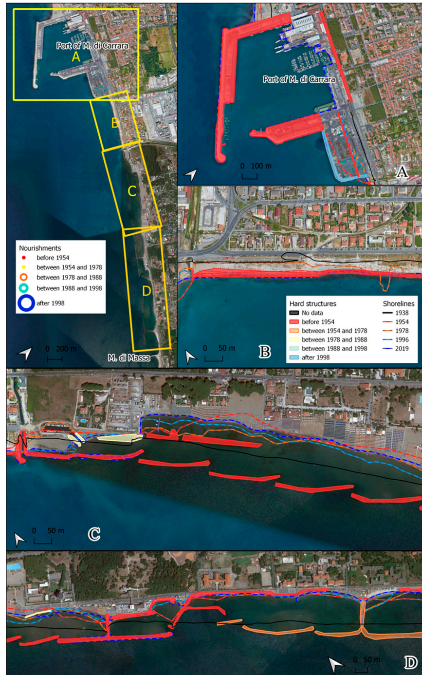
Figure 3. Identification of hard and soft operations along the sector comprised between the Port of Marina di Carrara and Marina di Massa. Polygons represent the hard structures; dots represent the nourishments. The yellow frames in the top left panel correspond to the zoom in panels to the right and at the bottom. The background image has been retrieved from the Google Earth database.
