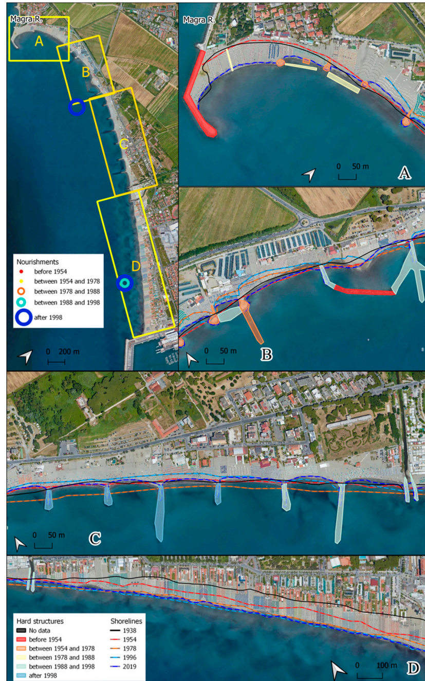
Figure 2. Identification of hard and soft operations along the sector comprised between the Magra River mouth and the Port of Marina di Carrara. Polygons represent the hard structures; dots represent the nourishments. The yellow frames in the top left panel correspond to the zoom in panels to the right and at the bottom. The background image has been retrieved from the Google Earth database.
