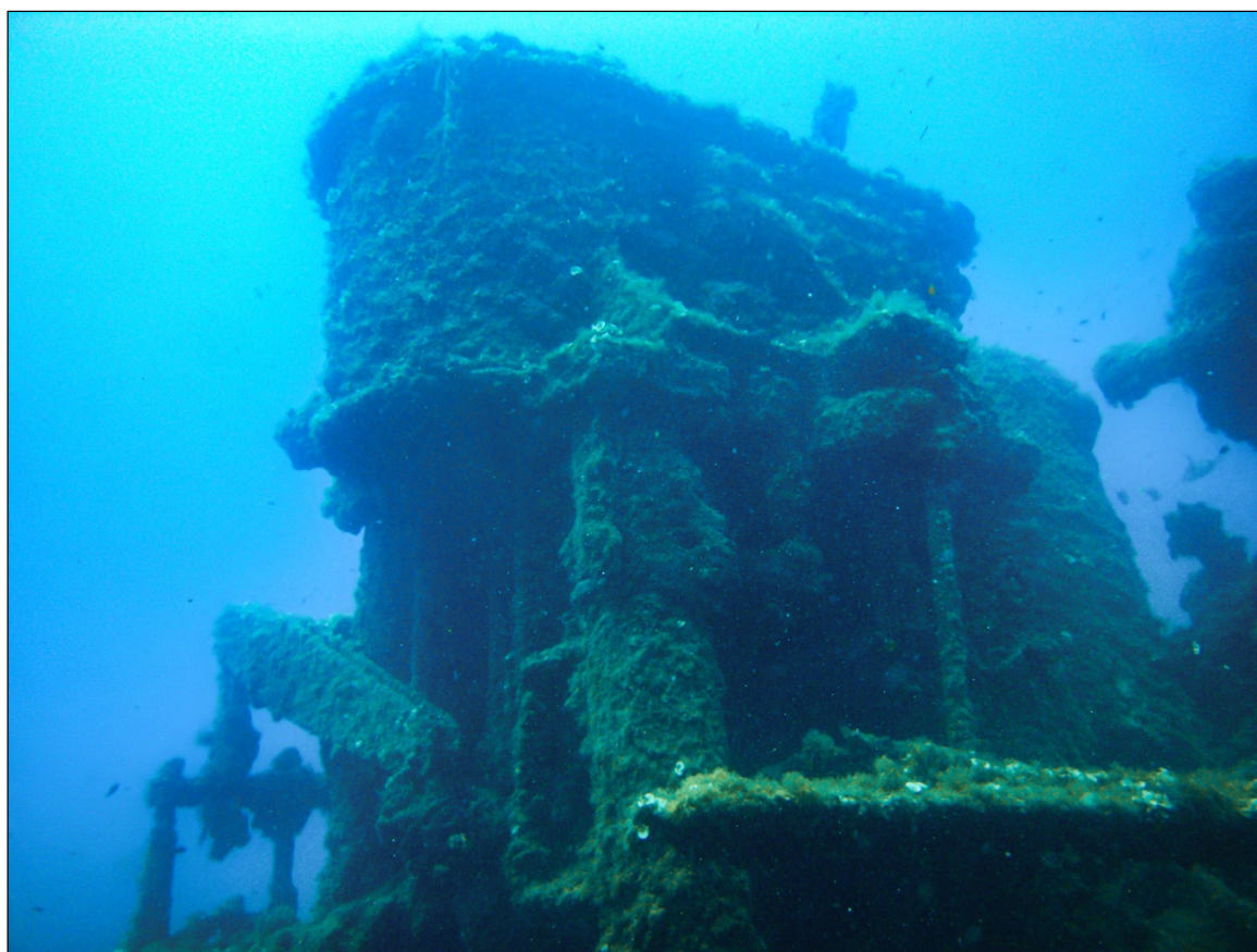
Figure 9. Wreck of the Bengala steamer. Detail of the huge compound engine of 254 NHP by “N. Odero and Ferro” of Sestri Ponente (Genoa) mounted in 1879 to replace the old engine of George Clark (photo credit: Salvatore Medaglia).
