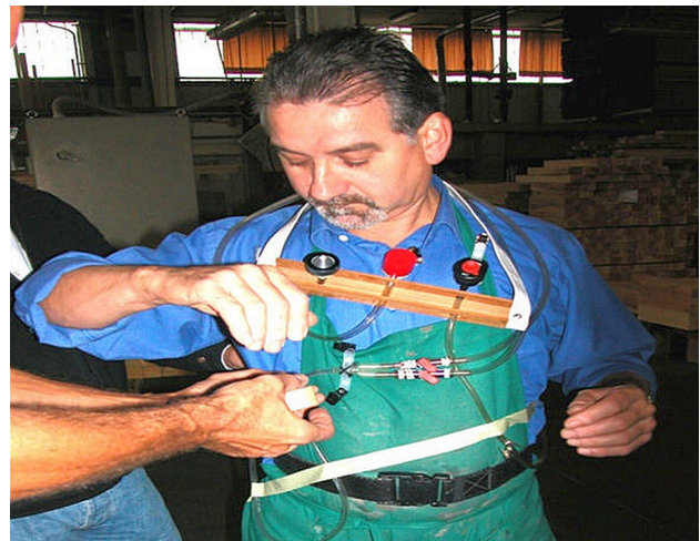
Fig. 1 Woodworker wearing three dust samplers (the IOM sampler at the left side of the subject) connected to the air sampling pumps
