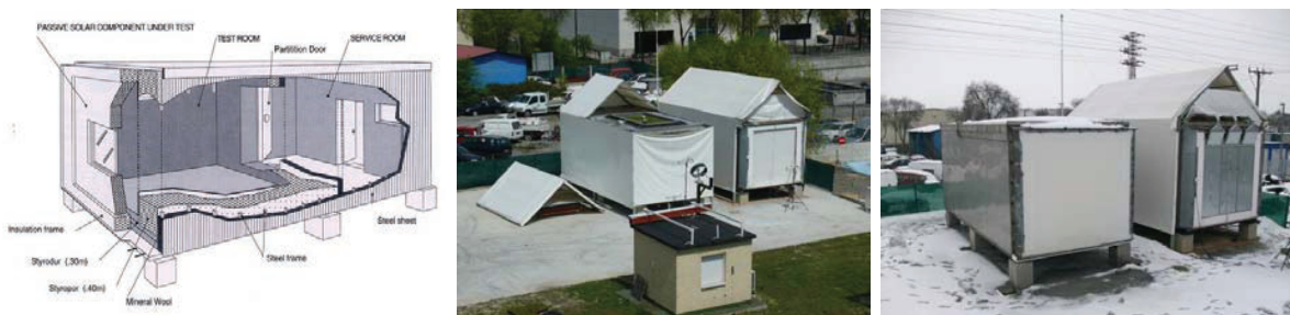
Fig. 1: (Left) Schematic of a PASSYS test cell (6). (Middle and right) Two PASLINK test cells in the Laboratory for the Quality Control of Buildings of the Basque Government, one of them also permits to test roof components.
