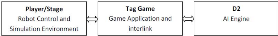
Fig. 2. Illustration of the three components of the framework; a robot controller (Player/Stage), an interlinking game application (Tag Game) and an AI engine (D2)
