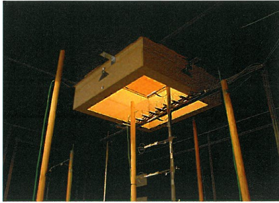
Figure 1: The inside view of the test room, the horizontal opening of S = 0.8 m, L = 0.4 m and L/D = 0.443 .
