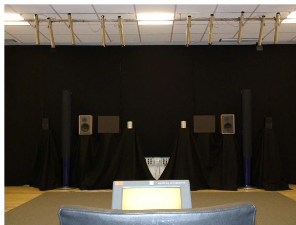
Fig. 7: Photograph of the setup (room fully illuminated). The fake wall is covered with a black cloth. The spot lights that illuminate the loudspeakers during the experiment are also visible. In the foreground, the chair for the subject and the touch screen are shown. The loudspeaker cable connections were left visible for the sake of plausibility.
