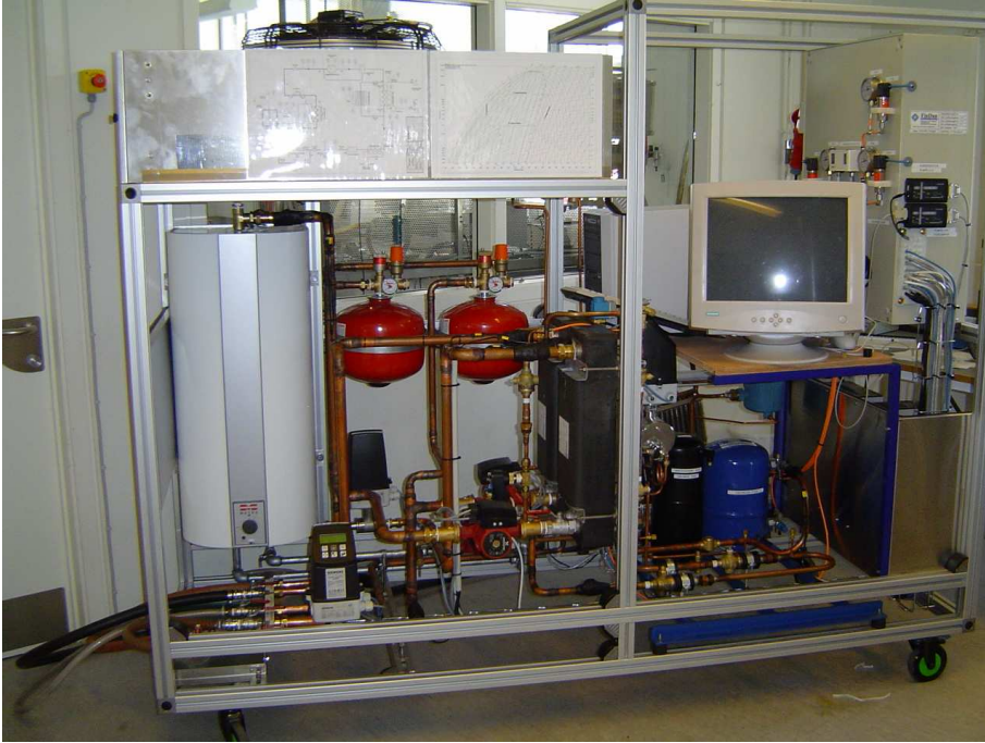
Figure A.11: Refrigeration test plant in Aalborg University
