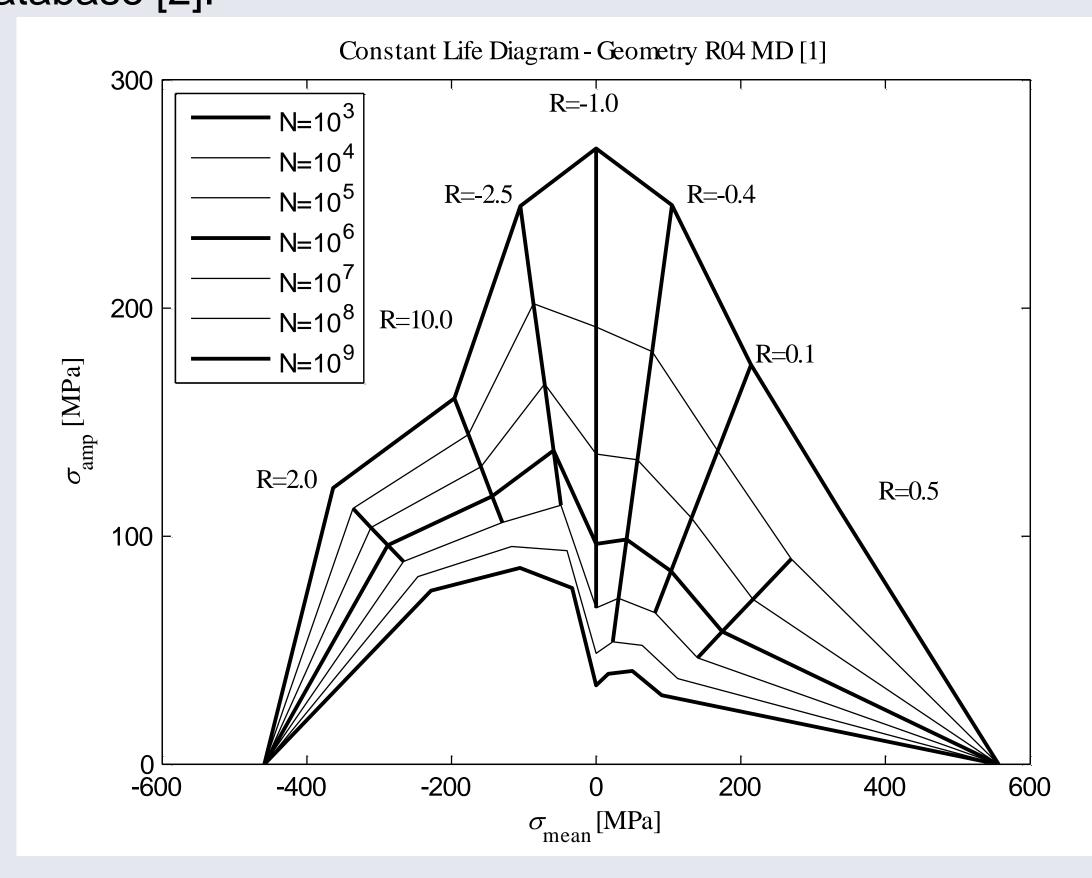
Damage accumulation from the individual load cycles has been widely considered in the literature and several models have been proposed. However, Miners rule for linear damage accumulation is still the most commonly used model in deterministic design, partly because of its simplicity and partly because none of the proposed models are superior. In the present paper the uncertainty on Miners rule is quantified based on variable amplitude coupon tests from the OptiDAT database [2].
