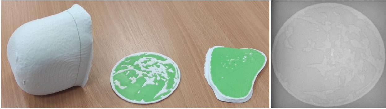
Figure 8. Printed breast phantom and two printed slices. The radiography image on the right is the x-ray image of the slice, shown in the middle.
