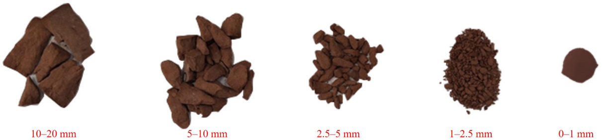
Fig. 8. The crashed fragments of a sample after SHPB impact.
