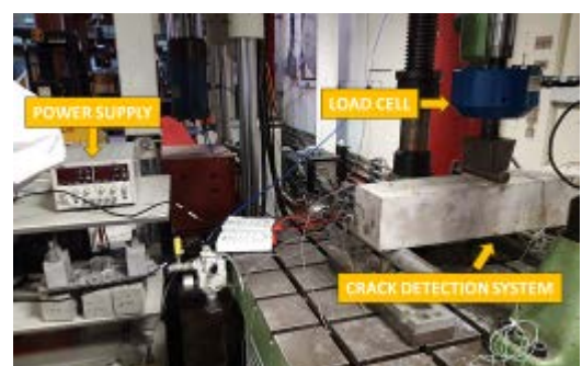
Fig. 5. Three-point bending test apparatus.
