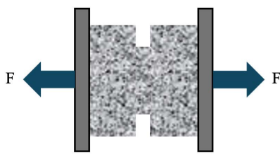
Specimen dimensions = 100x100x100mm 3 Notch depth = 25mm
