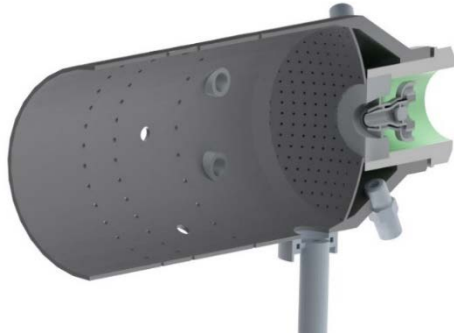
Fig. 1. RQL combustor atomiser and combustion chamber design.
