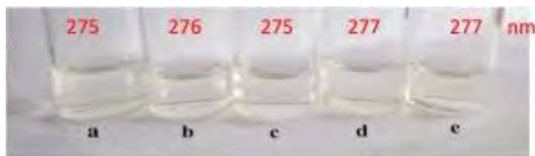
Fig. 3. Photos of NBP after UV exposure for different times (h):1 (a), 2 (b), 3 (c), 6 (d) and 12 (e). The UV absorbance maximum of each sample is showed in the upper series
