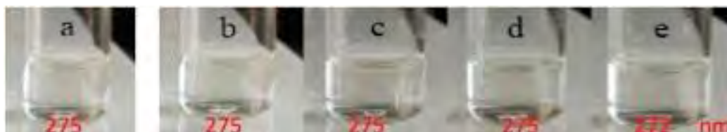
Fig. 2. Photos of NBP under various temperatures: at room temperature (a), 303 K (b), 313 K(c), 323 K(d) and 333 K (e). The UV absorbance maximum of each sample is showed in the lower series
