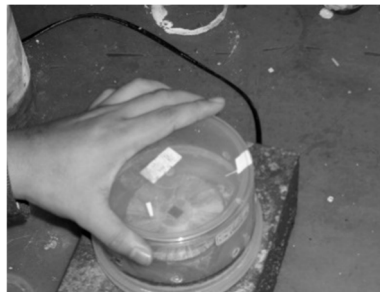
Figure 2. Process Growing the Ba_{0.5}Sr_{0.5}TiO_3 Film Doped with RuO_2 .
