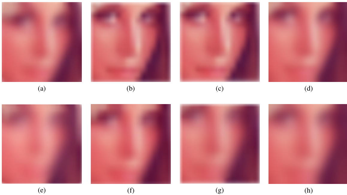
Figure 8: Blur techniques with the highest performance: (a) basic analysis and two-steps-forward-one-step-back synthesis using Safari; basic analysis and biquadratic B-spline synthesis using (b) Chrome and (c) Firefox; (d) for comparison an approximation to a Gaussian filter using an IIR filter [YvV95]. Blur techniques producing the best image quality: (e) wide analysis filter and two-steps-forward-one-step-back synthesis using Safari; wide analysis filter and biquadratic B-spline synthesis using (f) Chrome and (g) Firefox; (h) for comparison a wider IIR filter.
