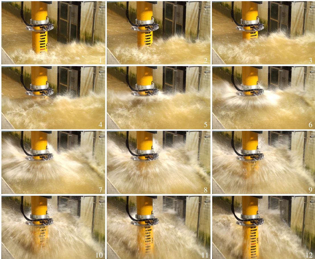
Figure 13. Pictures ( \Delta t = 0.08 s) of impacting irregular wave on solid platform (porosity 0%) at level +1.75. Maximum load 2.3 kN for h = 3 m, H_{m0} = 1.0 m and T_p = 5.9 s, all values in model scale.
