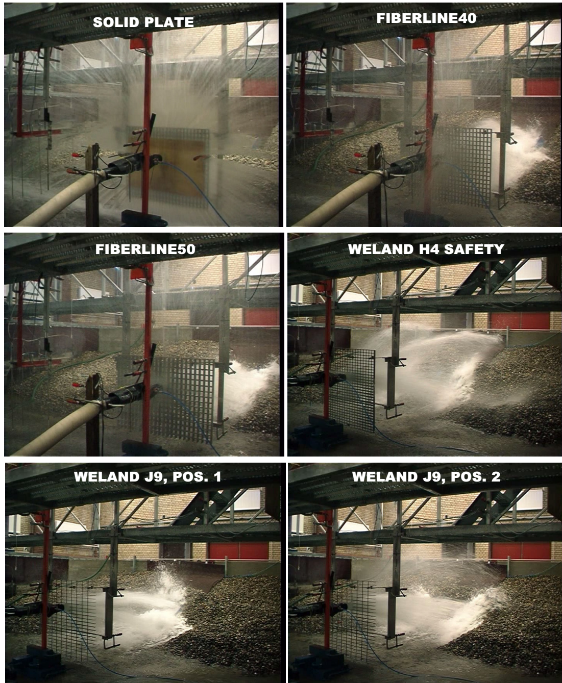
Figure 7. Pictures of perpendicular impact on the solid plate and the three different grates for close to identical jet velocities and no air added.
