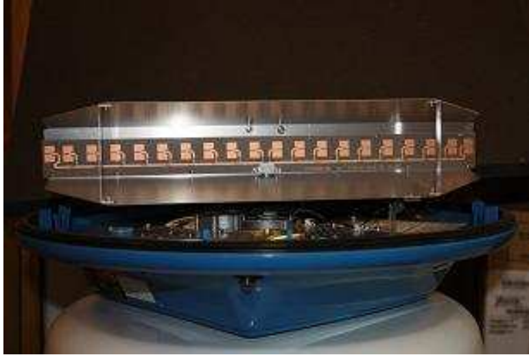
FIG. 2. Furuno 1715 with patched array antenna.
