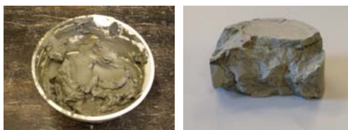
Figure 3: Homogenised soil used for the classification tests (left) and traversed dried soil specimen used in the first consolidation test (right).
