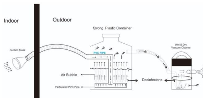
**Figure 2.** Example of modification on the concept of vacuum cleaner to reduce the aerosol. (Originally designed by Dr. AP. Hudyono).
