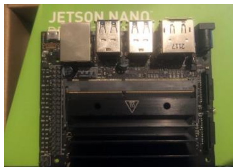
Figure 7 Jetson Nano: The mini-computer
