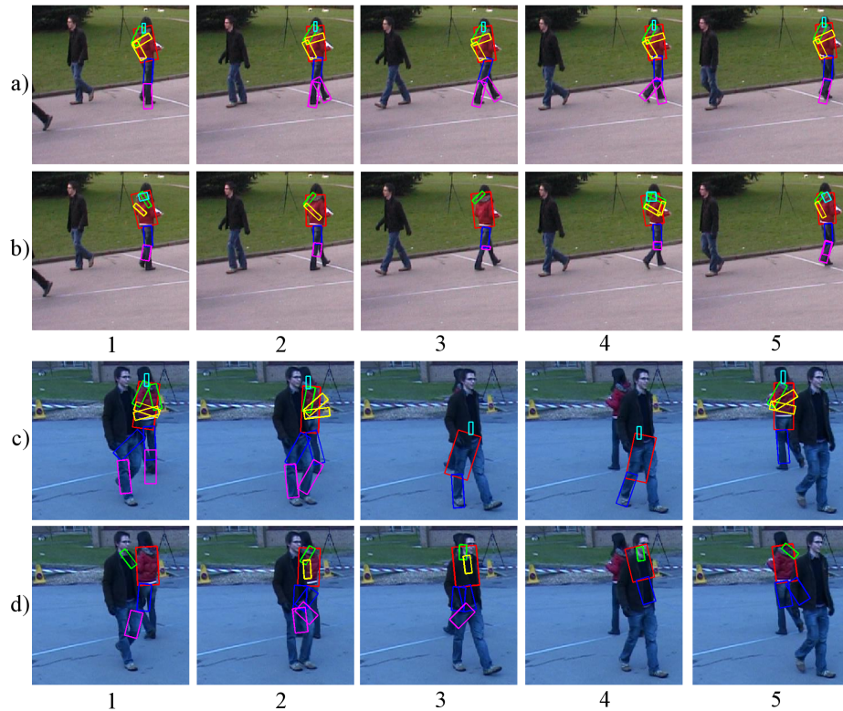
Fig. 4. Comparison of the multi-view approach against the single-view approach. Rows a) and c) show the results of pose estimation with the single-view approach. Rows b) and d) show the results of pose estimation with the multi-view approach. Each column of the figure shows a frame from two synchronized cameras.
