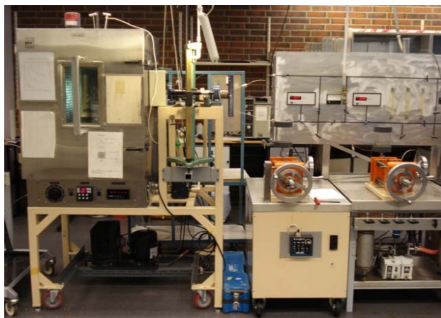
Fig. 4.3(a and b) An Actual photograph and Schematic diagram of JEFRI-DBR PVT system
