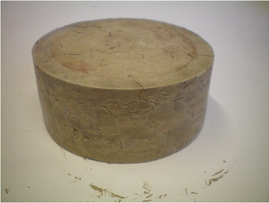
Figure 1: Fissured Søvind Marl after a consolidation test.
