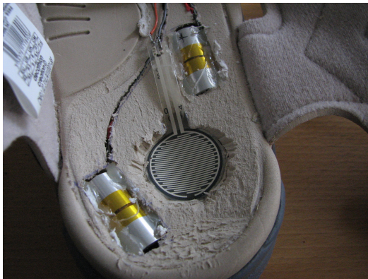
Fig. 2. A picture of one pressure sensor and two actuators embedded in the shoes.
