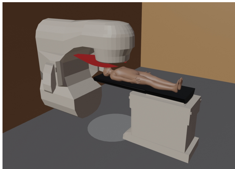
FIGURE 5.1: Screenshot of the Blender model including gantry and table stand in light grey, table top in black, laserguard in red and patient in skin color.
