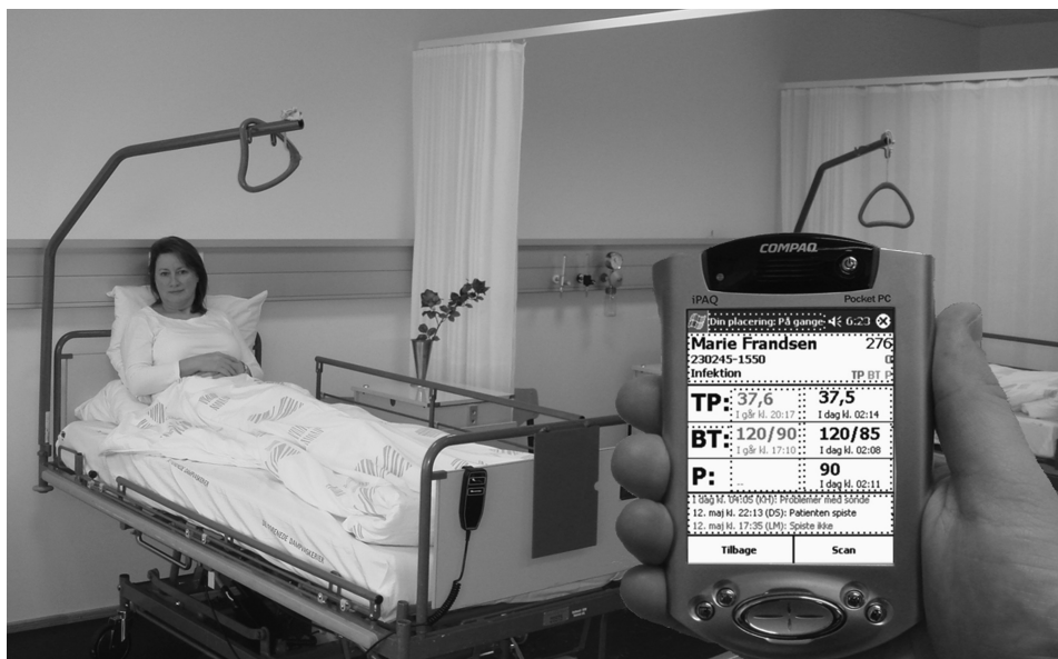
Fig. 6. MobileWARD prototype system: indexing patient information at a large regional hospital in Denmark to patients in proximity, location and upcoming work activities.
