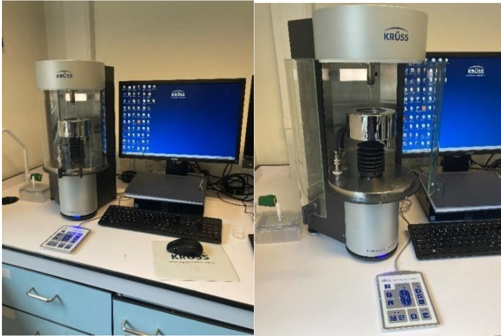
Figure 3-24: Photographic pictures of the BP100 maximum bubble pressure tensiometer taken in the KRÜSS lab.
