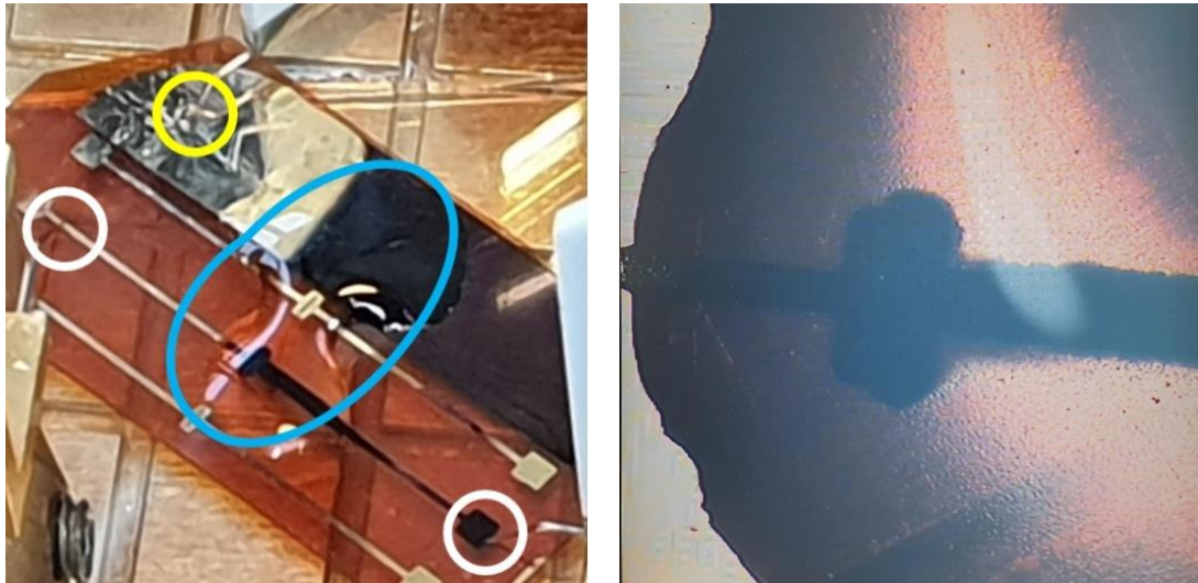
Figure 96 (left) Camera image showing probe station characterisation setup of PDTP-C4-acid OECT. 50 \mu\text{m} channel length. (blue oval) 20 \mu\text{L} of DPBS electrolyte solution overlapping PDTP-C4-acid thin-film and gold gate electrode. (white) biasing positions of source/drain (yellow) biasing position of gate electrode. (right) Microscope image of DPBS electrolyte solution covering PDTP-C4-acid thin-film.
