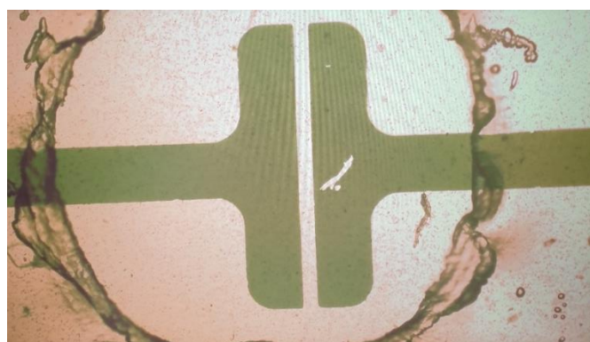
Figure 98 Polyimide tape isolated source-drain electrodes. Centre electrodes within Biopunctured hole are exposed. Electrode edges are insulated with polyimide tape.
