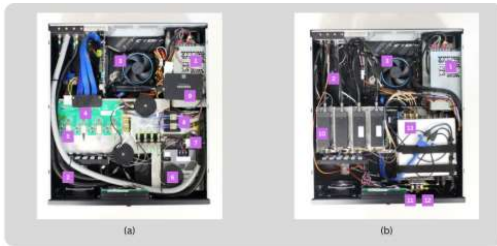
Fig. 2. (a) Alice QKD transmitter chassis (QRNG elements mounted below custom PCB). (b) Bob QKD receiver chassis. The elements highlighted in the figure are (1) power supplies, (2) optic fiber cables, (3) mother boards, (4) SLED driver board, (5) SLEDs, (6) sync laser driver, (7) sync laser, (8) manual variable optical attenuators (VOAs), (9) QRNG file storage, (10) single photon detectors, (11) photo-detector for sync laser signal, (12) constant fraction discriminator circuit, (13) time taggers.
