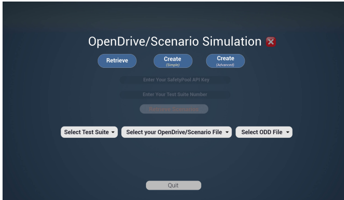
Fig. 7. Simulation GUI which shows the Retrieve, Create (Simple) and Create (Advanced) buttons for acquiring an OpenDRIVE/OpenSCENARIO file.
