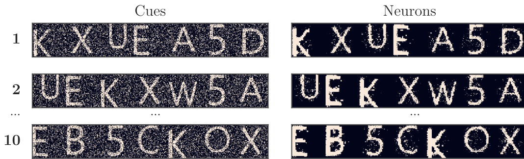
Fig. 7. Example of the SNAN test patterns from the general pretrained dataset (Fig. 4). Three testing cycles are shown. (Left) Testing images with 20% “salt-and-pepper” noise. (Right) Cued recalls in the pyramidal neuronal layer. The averaged firing rate on the test time interval for each neuron is shown.
