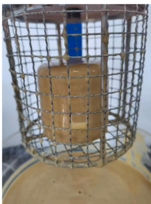
Fig. 12. Mudcake encapsulated by bentonite.
