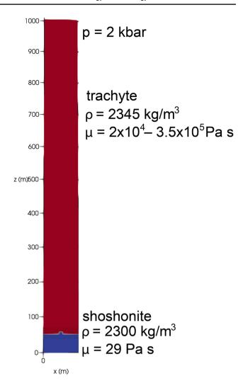
**Fig. 2** Setup for the simulations of magmatic interactions in the Zaro plumbing system. The small 2D vertically elongated reservoir contains trachyte (in red) and is intruded by shoshonite (in blue) from the bottom
