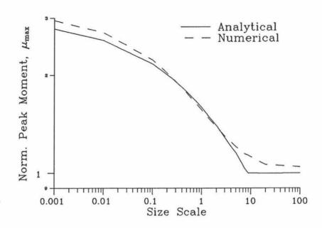
Fig. 9. Peak load at different size scales predicted by the model and by the DSS.
