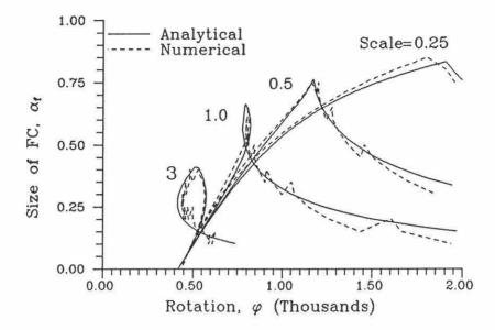
Fig. 7. Size of the fictitious crack for the analytical model and DSS. The loops are due to snap-back.
