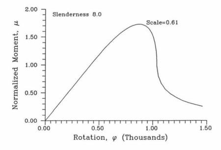
Fig. 10. Moment displacement curve for the beam on the critical size scale.
