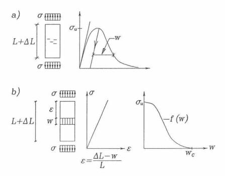
Fig. 1 a) Concrete rod subjected to uniaxial displacement controlled loading. b) In the fictitious crack model the displacement is divided into a stress-strain relation and a stress crack opening displacement relation.
