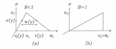
Fig. 3. Constitutive relation for the midsection of the layer a) When the layer is stable, B < 1.. b) When the layer is unstable B = 1.
