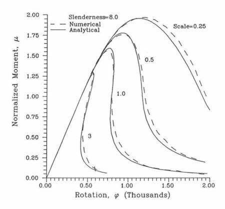
Fig. 6. Comparison between the analytical model and DSS using the standard beam at 4 different size scales.
