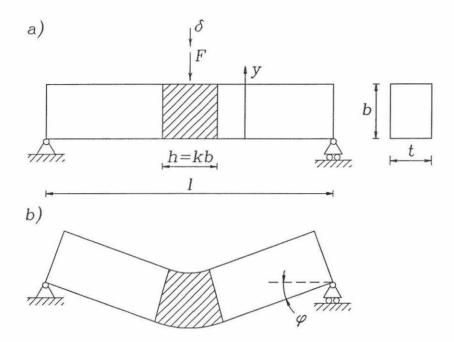
Fig. 2 a) The considered beam where the hatched area is the elastic layer. b) Deformed beam where only rigid body displacements are considered.
