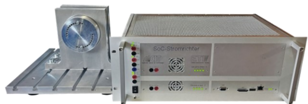
Fig. 9. Testbench with ETI – SoC System (right) [19], inverter [17] and the locked rotor testbench (left).
