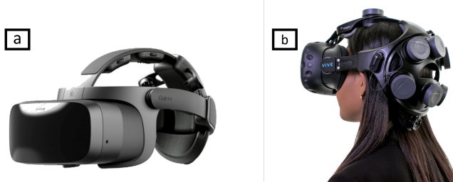
Fig. 1: Virtual Reality devices incorporating Electroencephalogram (EEG) readers: a) Galea VR headset with EEG sensors from Varjo/OpenBCI [5], b) BESA DSI-VR300 BCI integrated with HTC [6].
