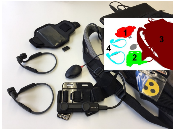
Figure 4.2.: The hardware of the prototype: (1) iPhone running the prototype app; (2) stereo camera for capturing objects in the environment and their distance to the user, fixed on GoPro chest straps; (3) backpack with a laptop on which the computer vision algorithm was running; (4) bone conduction headphones for audio output, one pair for the participant and one for the test leader (image ©Angela Constantinescu, Daniel Koester)
