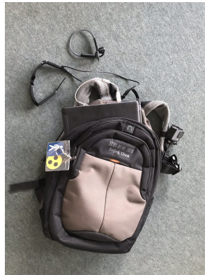
Figure 5.2.: Hardware of the sonification prototype without iPhone: backpack with laptop, sunglasses with small integrated camera, bone conducting headphones.
