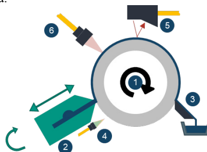
Figure 3: Setup with components – (1) High precision roll; (2) slot-die; (3) doctor blade; (4) gap sensor; (5) 2D-triangulation sensor; (6) line scan camera
