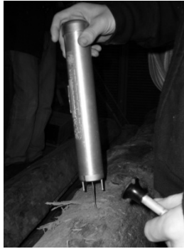
Figure 2.7: Pilodyn device and an example of its use
