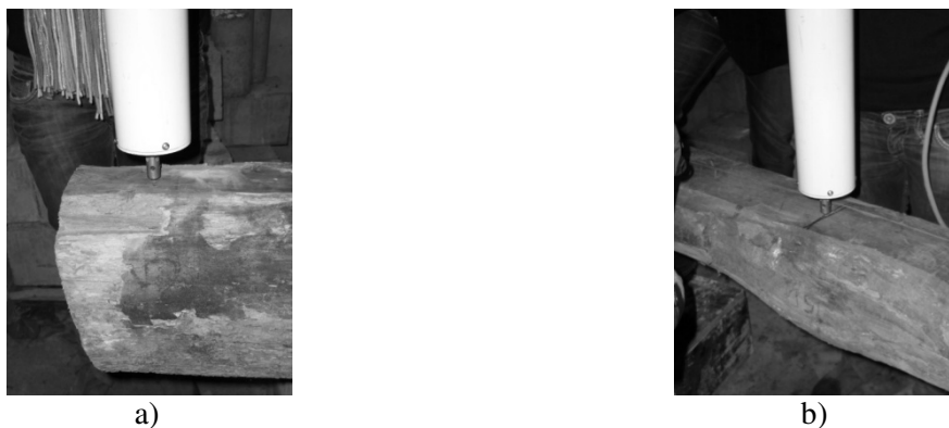
Figure 2.6: Resistograph use in a) top section b) middle section
