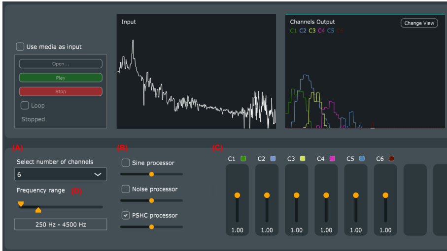
Fig. D.1: Screenshot of the application in action with a microphone as input source device. The upper section of the layout consists of two displays, visualizing the frequency spectrum of the raw input and processed output; with each channel displayed individually in the output spectrum. The lower section of the layout constitute the user-configurable parameters, and can be modified to adjust the output in real-time. Use (A) to select number of channels, (B) to enable and disable carrier types, and control the gain of each carrier, (C) to control the gain of each individual channel, and (D) to adjust the upper and lower cut-offs of the frequency range in which the band-pass filters will be distributed between.
