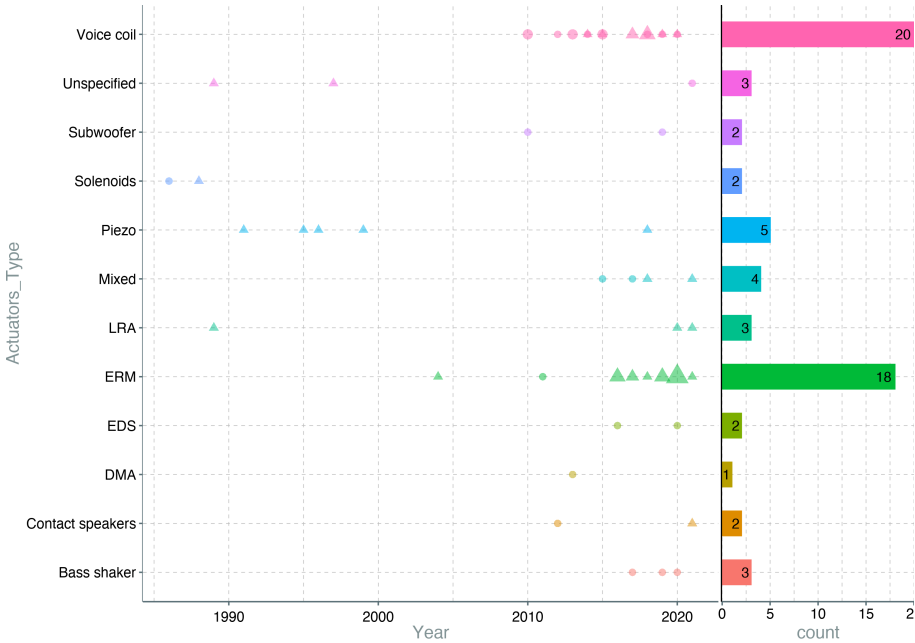
Fig. A.4: Distribution of types of actuators used over time; a triangle indicate a wearable device, a circle indicates a fixed device and the size of the shape represents the amount of similar devices
