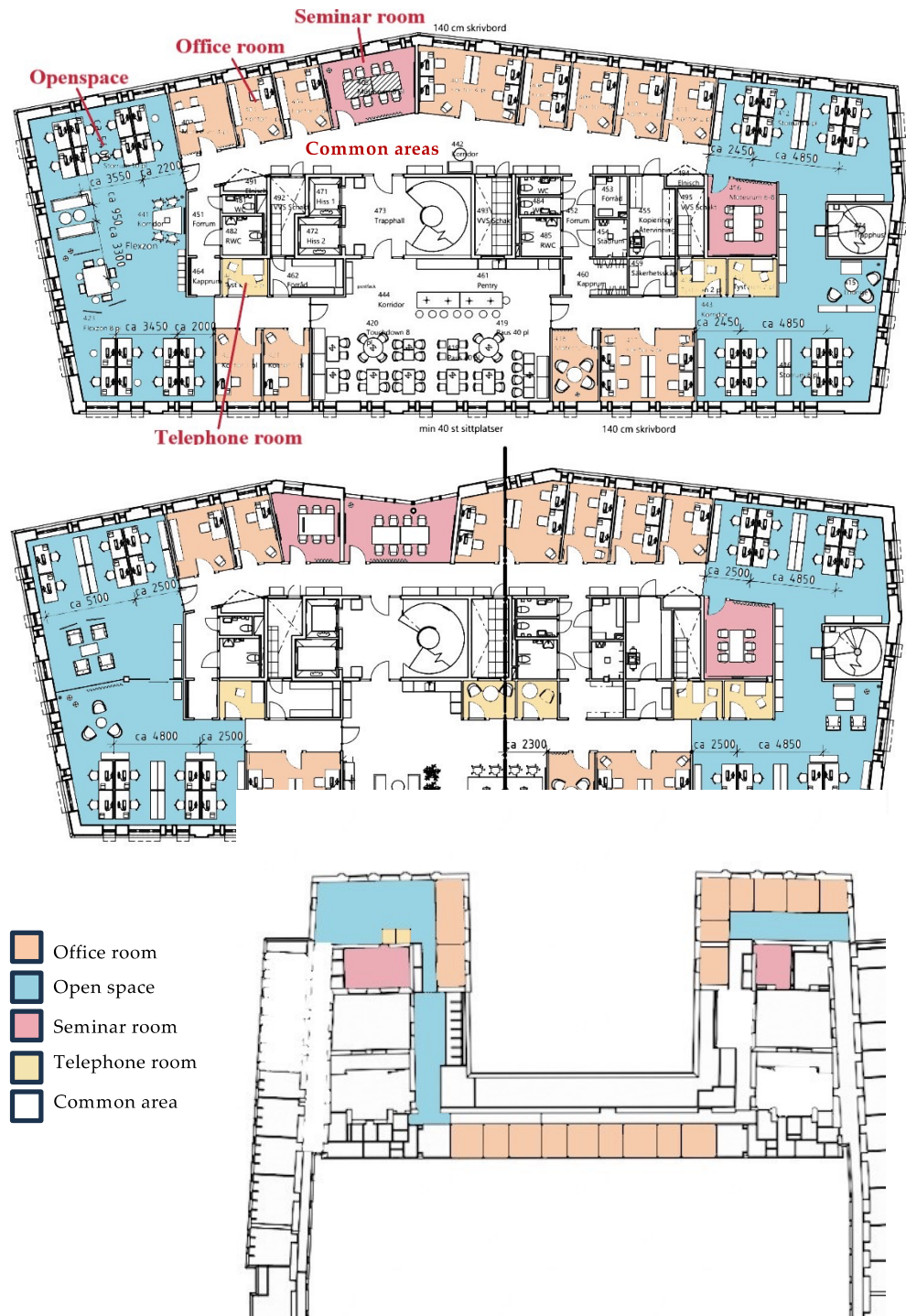
Figure 2. Floor plans of Department A (2 floors, top two floor plans) and Department B (bottom floor plan). Orange: office rooms. Blue: open spaces. Red: seminar rooms. Yellow: telephone rooms. White: Common areas such as corridors, kitchen, and toilets.
